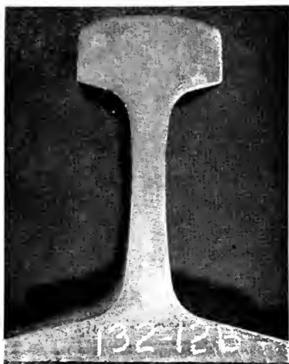
Fig. 8 (Investigation 132-12B)—Cross section of a rail that was cut through a point exhibiting an internal imperfection. This imperfection, detected by a Sperry detector car and hand test, can be noted in the web.
